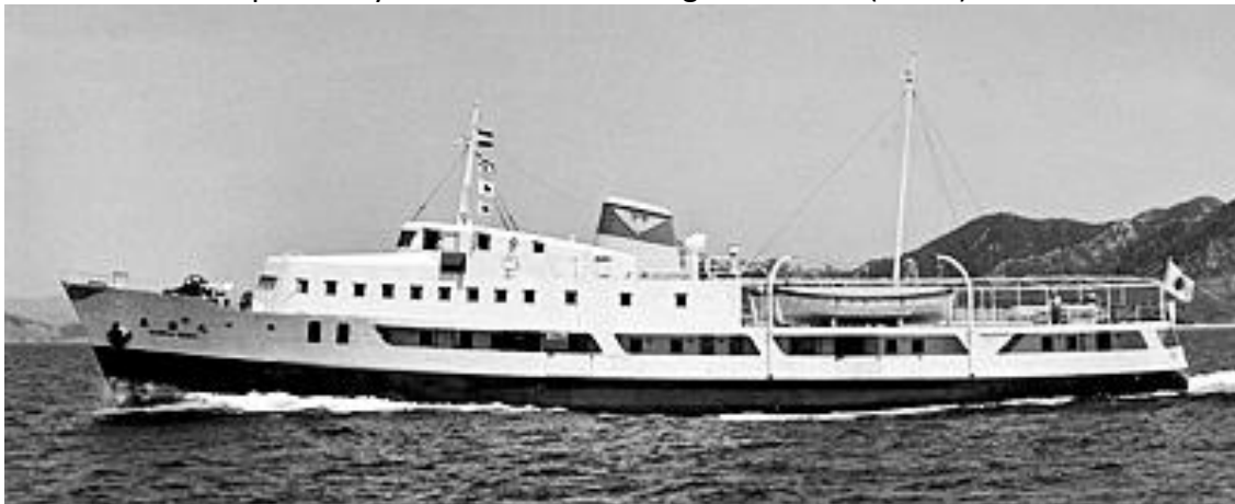
NANKAI MARU as built. Nice profile but open deck at stern allowed tragic ingress of water in typhoon (builders).
