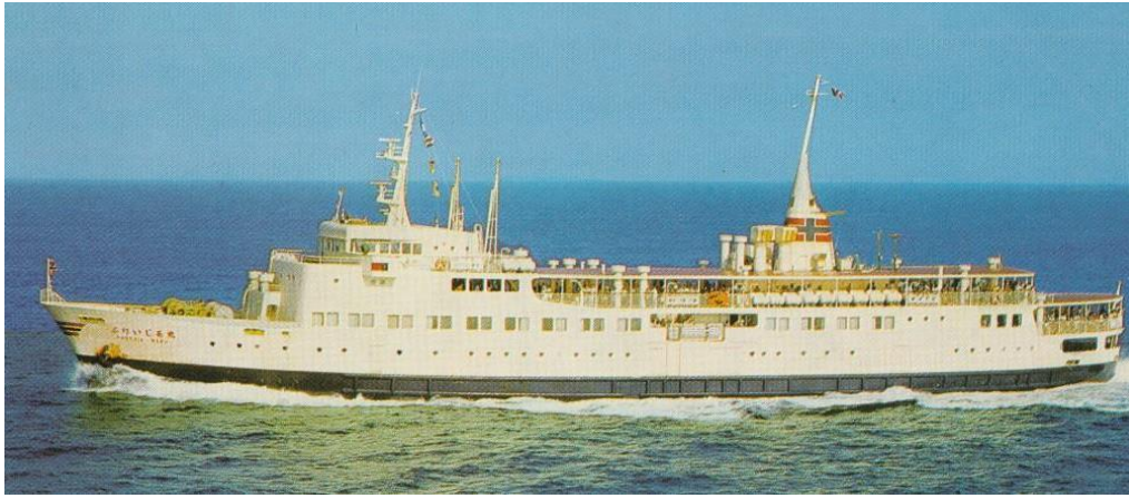
FREESIA MARU, unusual fender and vertical blocks (from a Tokai Kisen postcard).
