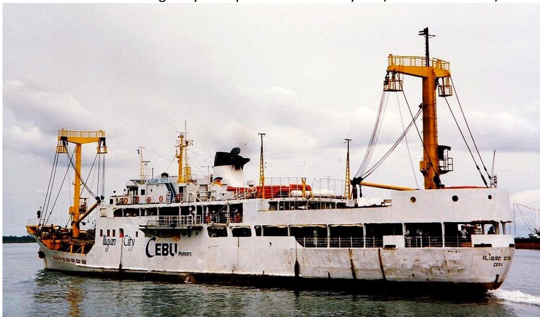
As ILIGAN CITY in Cebu Ferries colours with new masts and modified superstructure, mid-1996 (Howard Dick*).
